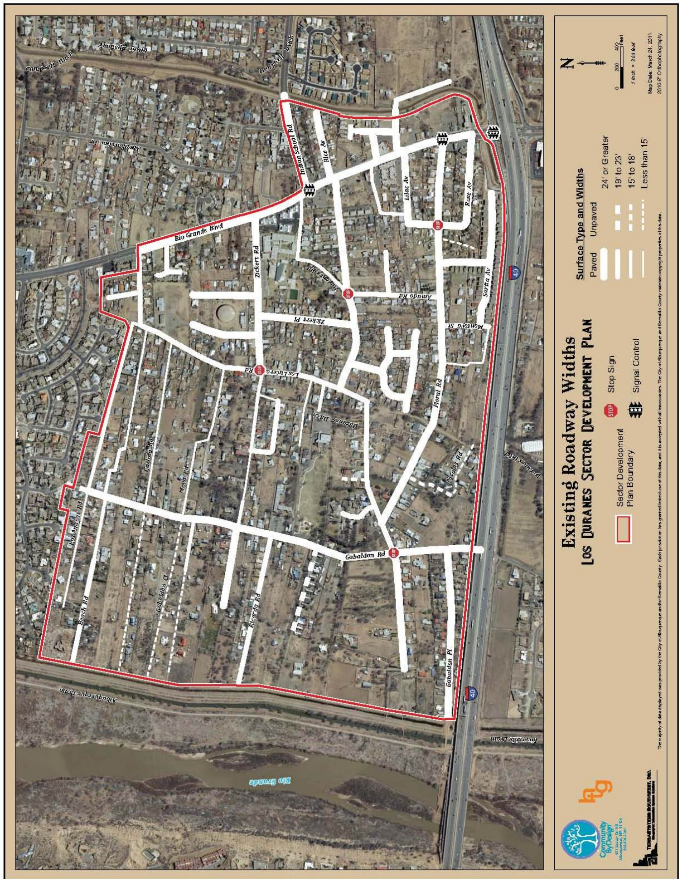
Figure R Roadway Widths
