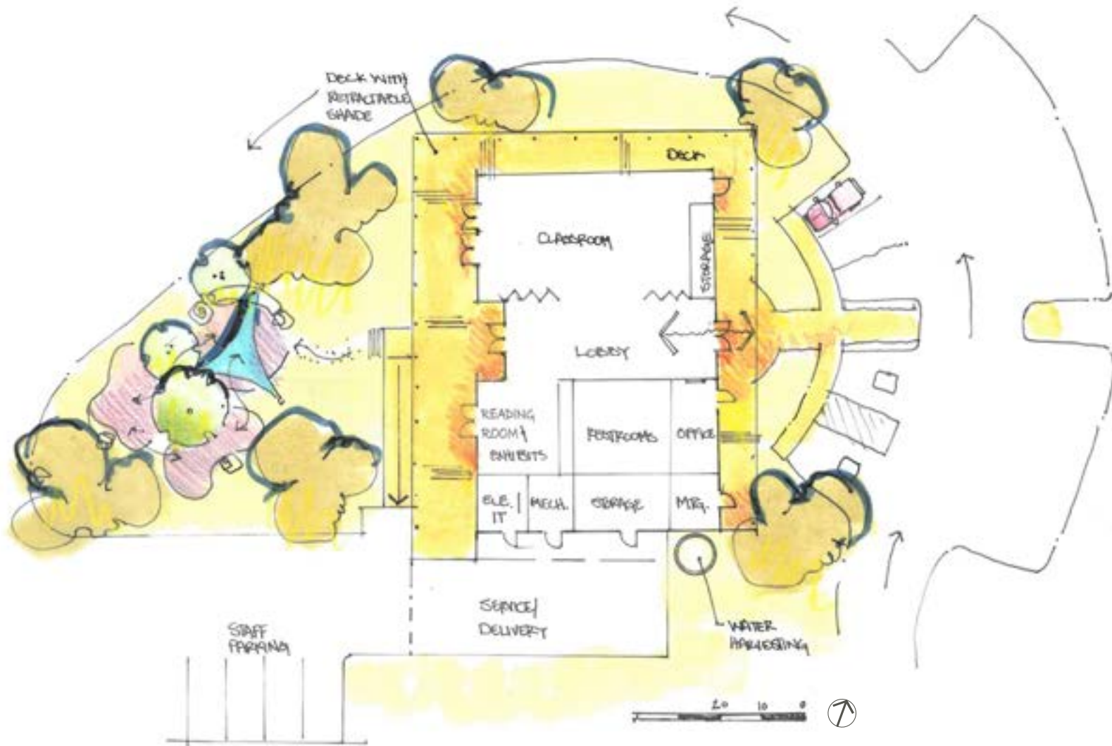
FIGURE 13. SITE 3 PARKING AND CIRCULATION AND PRELIMINARY FLOORPLAN
