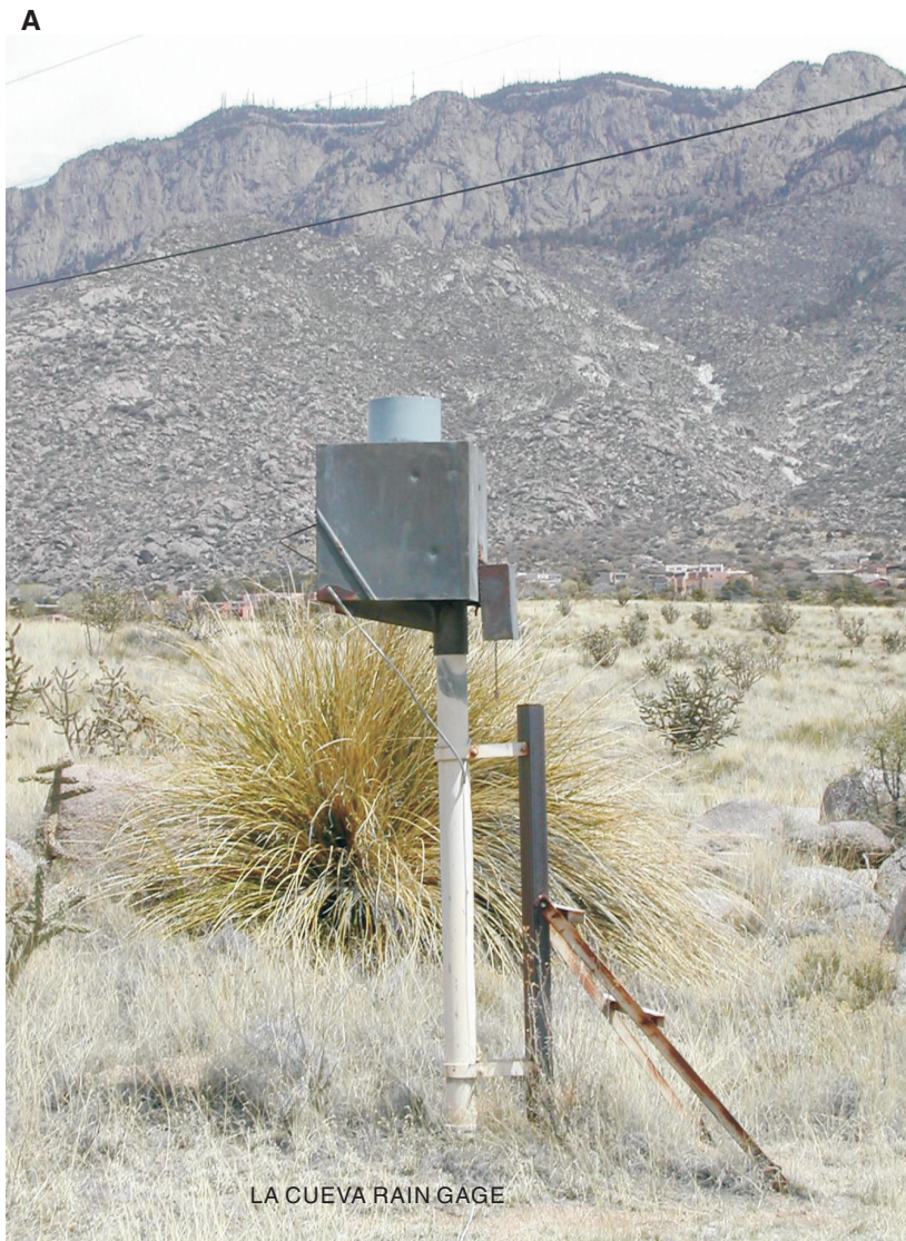
Figure 2. (A) La Cueva rain gage, (B) recorder next to rain gage, and (C) view inside of rain gage.
