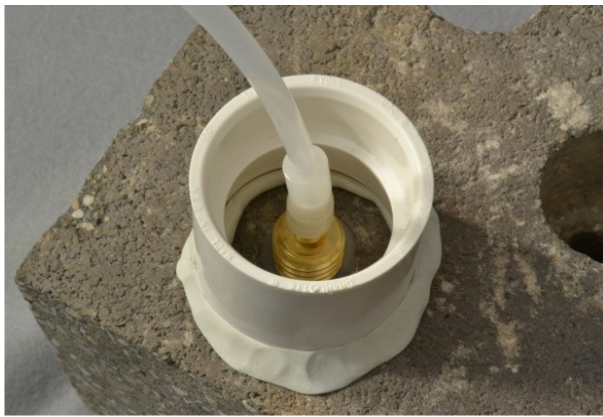
Figure 6. Water dam used for leak detection.
