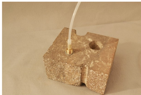
Figure 5. Vapor Pin™ sample connection.
