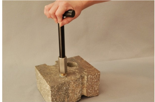
Figure 7. Removing the Vapor Pin™.
