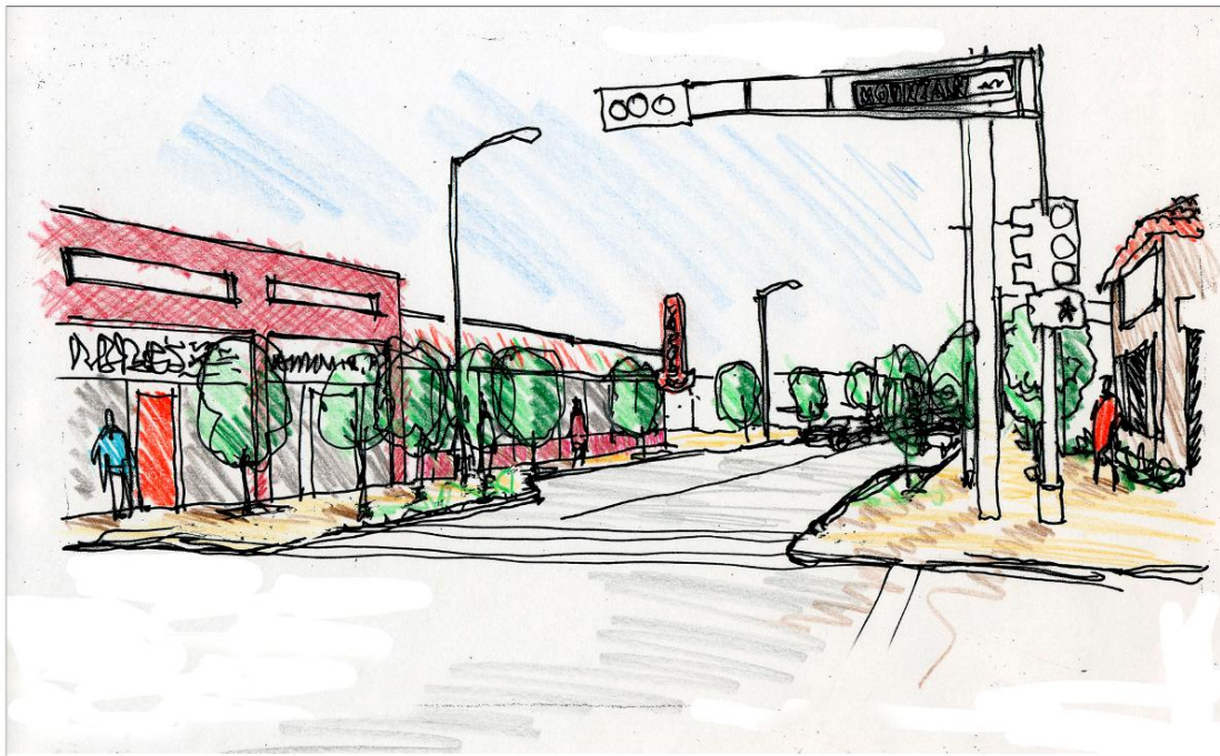
“Bump-outs” may also be created at major intersections. These “bump-outs” serve to define the intersections while shortening the distance pedestrians must travel to cross the street.
